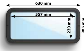
Rounded corners (r=60 mm), excellent insulative value
