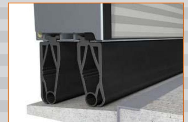
For enhanced energy retention Alpha uses a double rubber profile on the ISO 80 Door with an inward curved sealing lip for optimum sealing. The rubber profiles are accommodated by a special plastic profile with a low heat conduction, furthermore the sealing lip of the rubber profile forms a tight connection with the vertical lateral seals.
